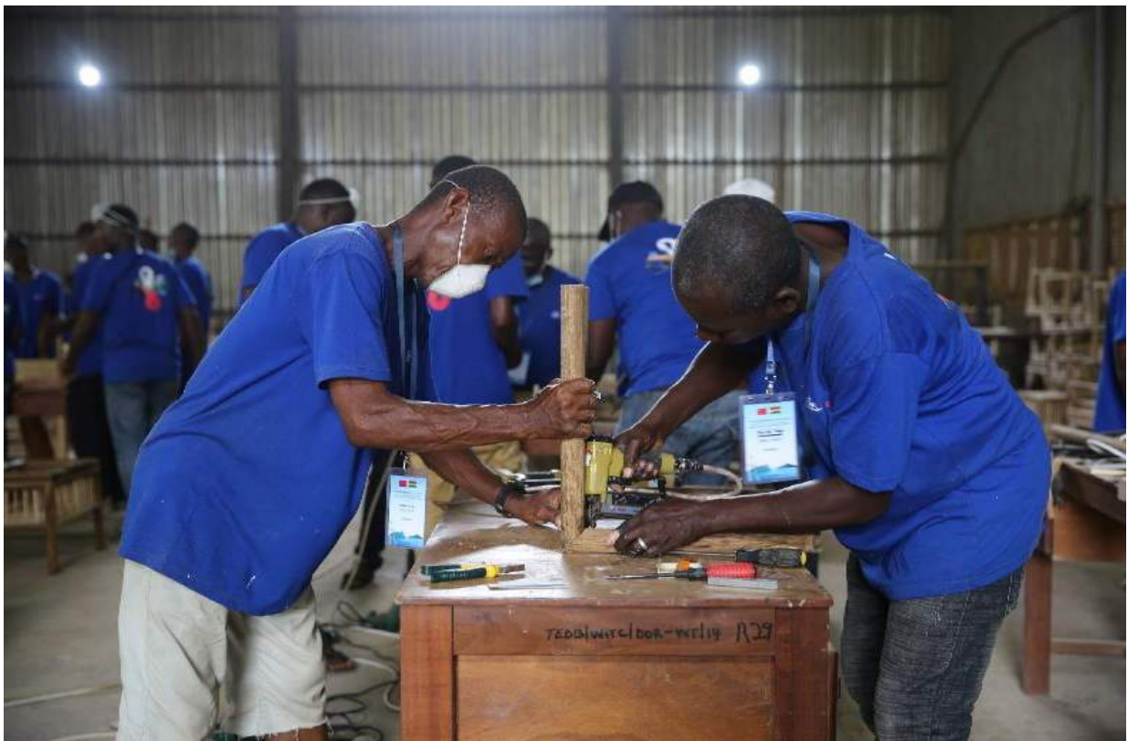
Fig 79. The picture above shows some artisans putting bamboo joints together to construct a coffee table with the aid of a shooting gun.
