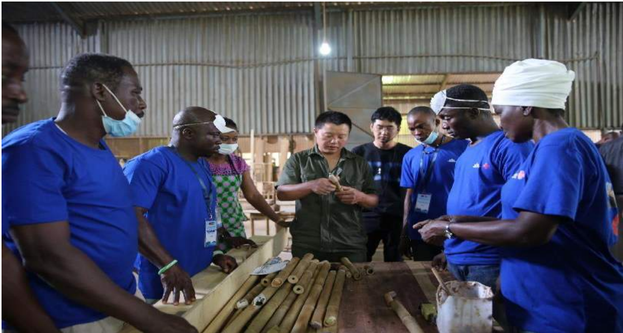
Fig 74 shows a resource person demonstrating how to insert the round wood into the bamboo culms in order to join the culms together to produce a table
